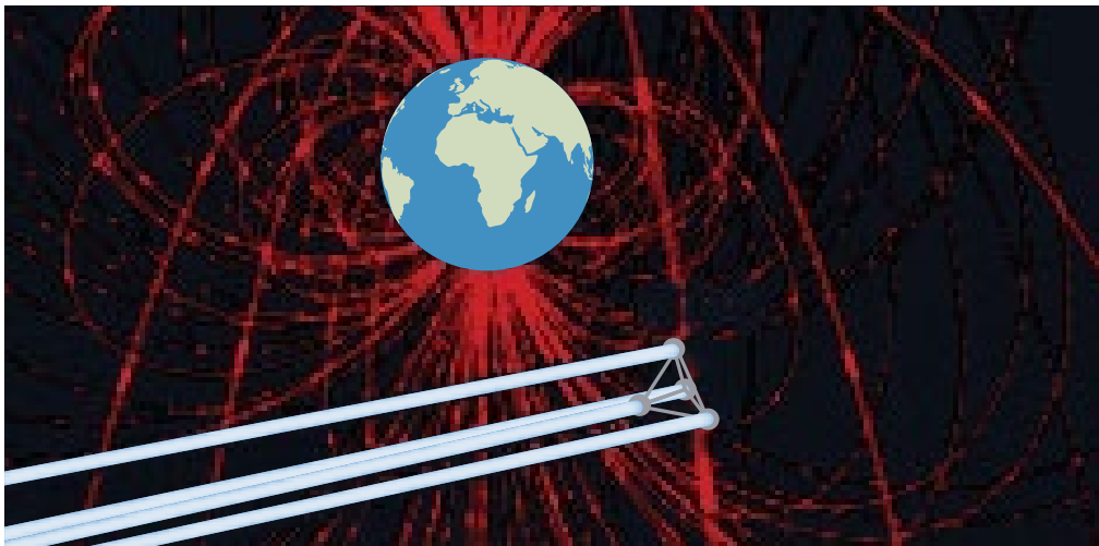
Figure 4.10. The four MMS satellites flying in formation. Tetrahedral pattern is used to capture the 3D structure of the encountered reconnection sites.
